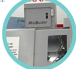
**Pedestal stand** unit is mounted on a floor stand and ducted to a machine tool.
